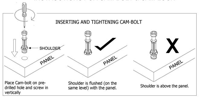
Place Cam-bolt on the designated pre-drilled holes on the panel. Use a Phillips Screwdriver to screw-in Cam-bolt vertically until shoulder is flushed (on the same level) with panel.
