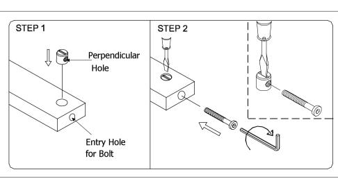
Use a Flathead Screwdriver to hold Barrel Nut in position before inserting bolt to thread into the Barrel Nut.
