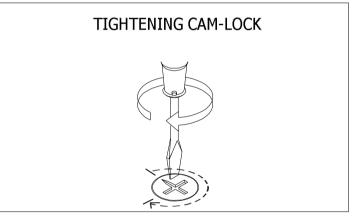
Use a Flat-head Screwdriver to turn Cam-lock clockwise so it locks onto the head of the Cambolt. Turn until it is snug (about 3/4ths of a turn) -- over-tightening could damage Cam-lock or/and Cam-bolt.
