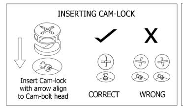
Align the arrow on the Cam-lock to the Cambolt head and insert the Cam-lock. Ensure Camlock is fully inserted.
